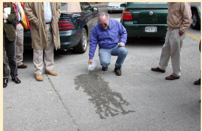
Figure 4. Visual inspection of a pervious concrete lot in Georgia shows accumulation of both sediment and leaf debris (left). The fact that the lot is clogged is confirmed by emptying approximately 1 gallon of water on the lot, which subsequently runs off rather than infiltrating (right).
