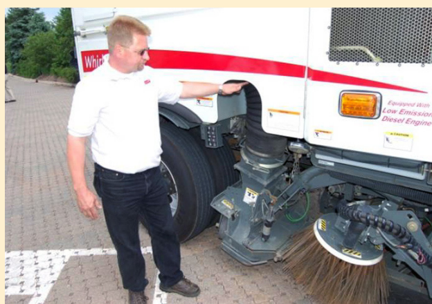
Figure 5. A small mechanical street sweeper (top) and the underpinnings of a vacuum sweeper (bottom).
