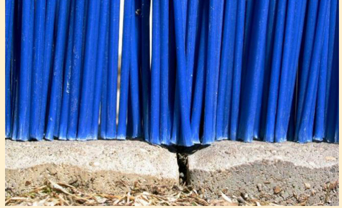
Figure 6. Mechanical sweeper bristle penetration of larger gaps associated with CGP filled with sand (left) is possible, but pavement types with small gaps (such as PICP) is not (right, courtesy of Elgin Street Sweepers).
